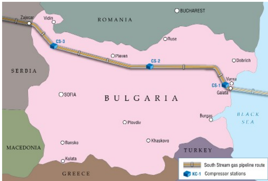
South Stream project layout in Bulgaria
